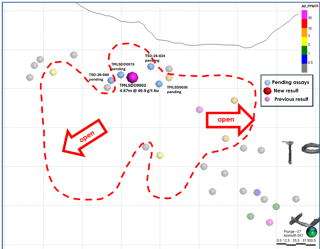
Figure 5. Oblique section through the newly identified Fundoot Splay showing the high-grade discovery intersection, pending further assay drillholes, and open extensions along strike and down dip.
