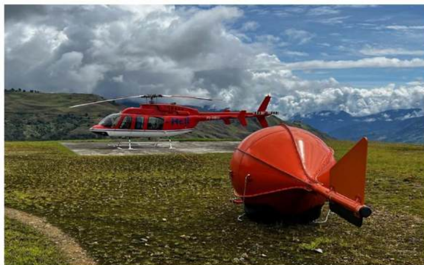
Figure 30 - Airborne MT Underway over Tolukuma, Helicopter and suspended array
